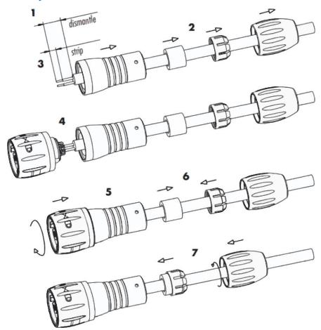
If a cable is already connected to the connector remember to unscrew the cable clamp before unscrewing the main body of the connector otherwise, you risk twisting the cable and breaking the connections. If the main body is difficult to unscrew it may be easier to lock the connector to the handheld then grip and unscrew the main body in an anti-clockwise direction.
