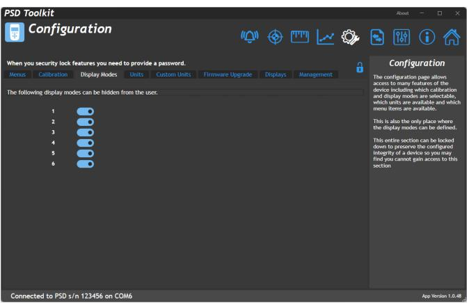
This section allows you to enable or disable the available six display modes from selection using the keypad (If that functionality has been configured)
