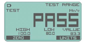
The High limit, Low limit and actual Value are displayed underneath. Soft keys allow for toggling between Zero and Gross and the Units can be selected.
