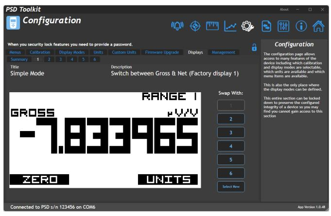
Configure the available Display Mode slots with the required Display Modes.
