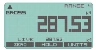
The other soft keys allow being able to Zero the main display or go back to displaying Gross. As usual there is a soft key to allow Units to be selected.
