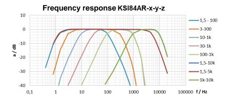
The HP filter of the **velocity** sensor types has a stopband attenuation of -50 dB/decade, the LP filter has a stopband attenuation of -40 dB/decade.
