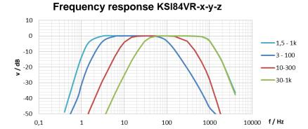
The HP filter of the **displacement** sensor types has a stopband attenuation of -60 dB/decade. The upper cut-off frequency is 300 Hz. It results from the significant decrease of the <u>dynamic range</u> with increasing frequency. At 300 Hz the maximum current amplitude is only 1 % of the <u>measuring range</u>.
