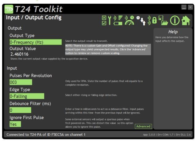
This module does not provide calibration, as such, because it is factory calibrated. However, on this page you can select the output type and parameters unique to your input sensor.
