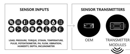
T24 transmitter modules collect data from industrial sensors including load, pressure, torque, strain, temperature, pulse, potentiometer & 4-20 mA / 0-10 V conditioned sensors. OEM PCB transmitters also available for integrated solutions.
