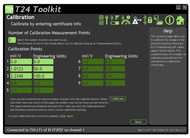
In some circumstances it may not be possible to apply inputs in which case the calibration can be entered manually from the calibration table or certificate for a load cell without ever having to connect the load cell.
