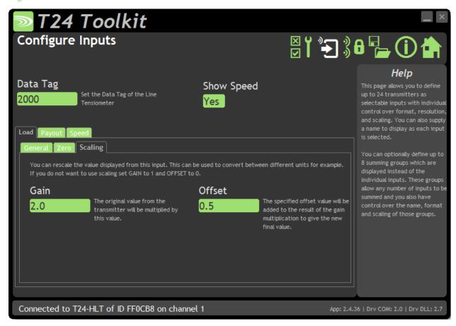
This page allows you to configure the channels with the use of a custom gain and offset. For the Load, Payout and Speed channels this allows displaying the values in different engineering units from those transmitted.
