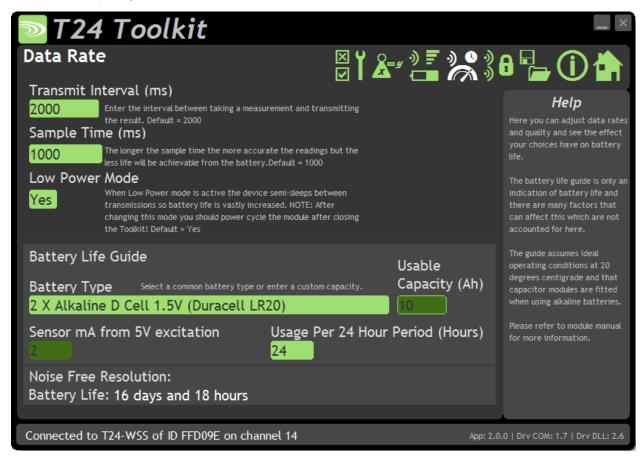
This page allows you to select the rate at which data is transmitted from the transmitter module and the quality. By selecting low power mode and entering some other information the toolkit will also give guides on achievable battery life.
