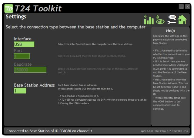
Select the appropriate interface type for the connected base station. If the base station is connected via a serial port then you will need to know the COM port it is connected to and the baud rate.
