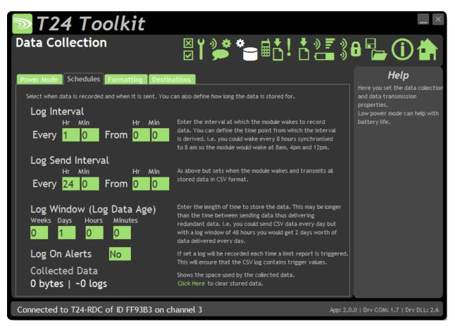
This tab sets the intervals at which data is collected and at which the CSV data is transmitted. This has an effect on battery life as in Low and Ultra Low Power modes the Log Interval determines how often the module wakes from a very low power sleep mode. See Battery Life section
