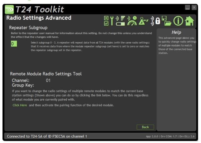
Here you can change the repeater subgroup settings for the connected module. Also a tool is provided to quickly match remote module radio settings to the base station radio settings.
