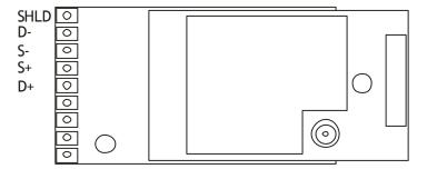
The Pt100 probe can be connected in 2, 3 or 4 wire measurement configurations.
