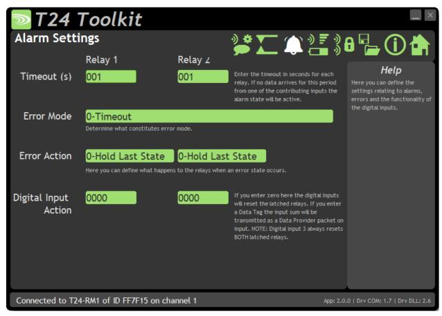
This page defines how the individual relays will react to time outs and errors present from any defined T24 module, as well as how Digital inputs 1 and 2 are used.
