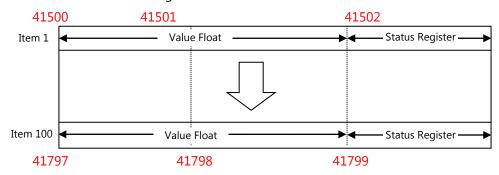
When reading registers containing the floating point data the register pairs must be read at the same time otherwise incorrect values could result because of partial updates during reading.
