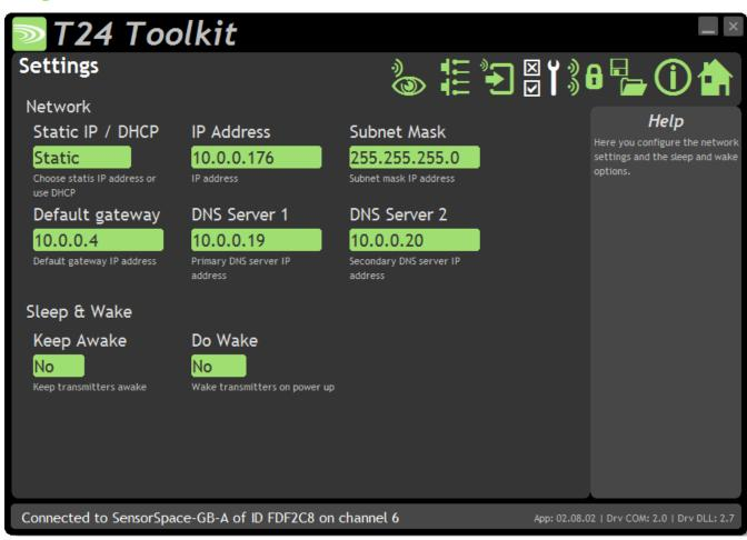
This page allows you to configure the Ethernet network settings and the wake functions.
