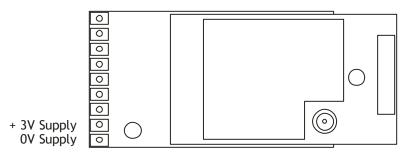
Connect to a 3 Volt power supply or batteries.
