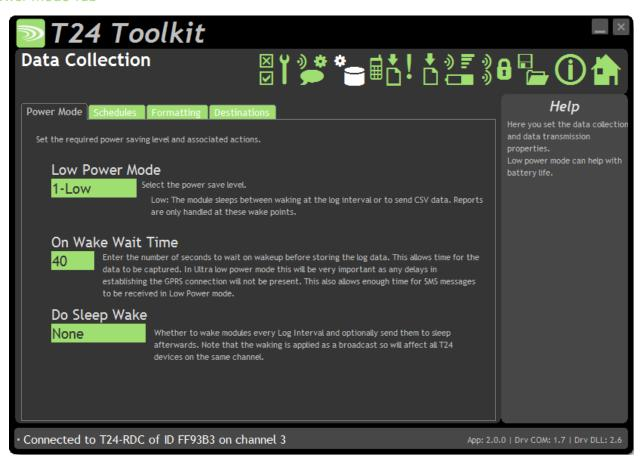
Here you define the how the data is collected and when and also determine how the CSV file is formatted and where it is delivered to. The Power Mode tab lets us change the following.
