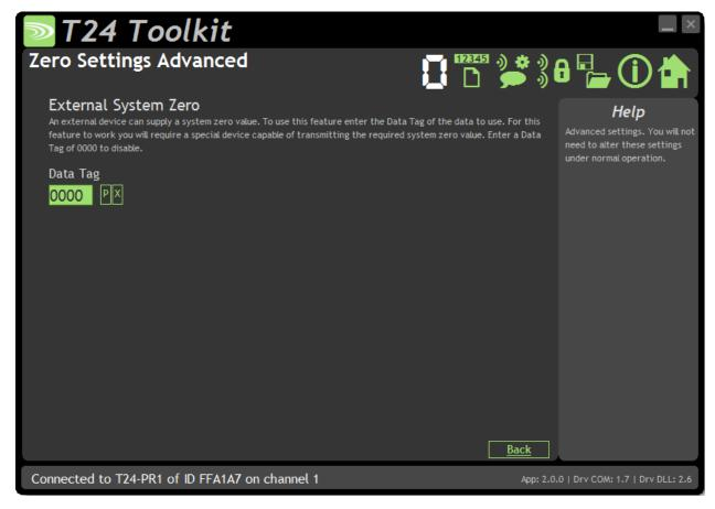
This advanced section allows the use of a specially configured external module to supply the system zero value for the handheld to use.
