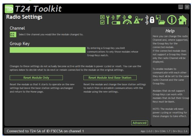
Here you can change the channel and group key for the connected module.
