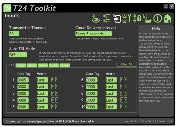
Here you can set timeouts and specify transmitters and also choose the interval between deliveries of data to the cloud platform.
