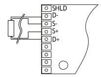
The four-wire resistance thermometer configuration increases the accuracy and reliability of the resistance being measured: the resistance error due to lead wire resistance is zero. In the diagram above a standard two-terminal RTD is used with another pair of wires to form an additional loop that cancels out the lead resistance. It provides full cancellation of spurious effects; cable resistance of up to 15 ohms can be handled.
