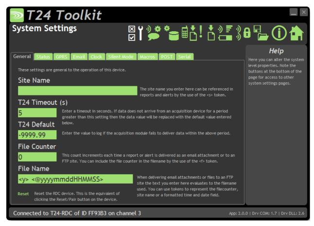
This is where much of the operation settings are configured. The parameters are split over multiple tabs. Just click a tab to move to the desired section.
