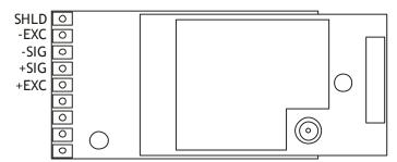
The resistance of the strain gauge can be between 85 and 5000 ohms. The T24-SAf can support up to 4 350 ohm strain gauges bridges attached in parallel (At the expense of reduced battery life).
