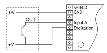
Onboard resistor configured for pull down and suitable excitation voltage selected
