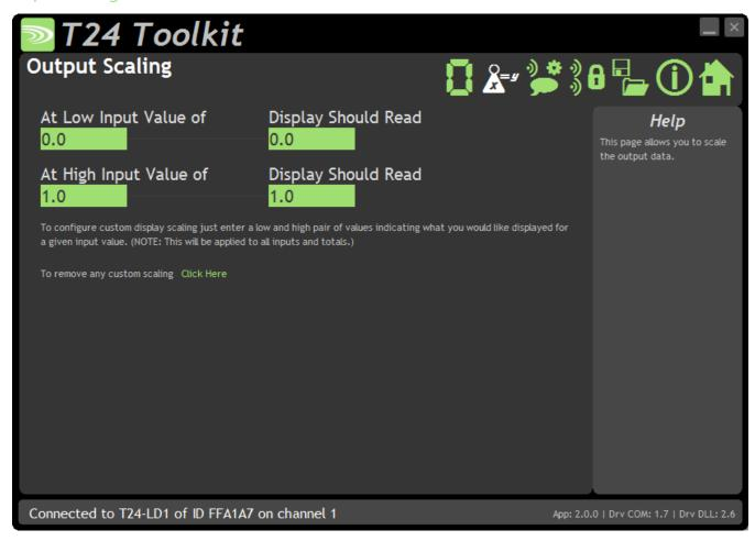
Use this page to scale the data displayed on the T24-LD1. This may be used, for example, to convert the data from a transmitter module calibrated in kg so that the T24-LD1 display shows the value in tonnes.
