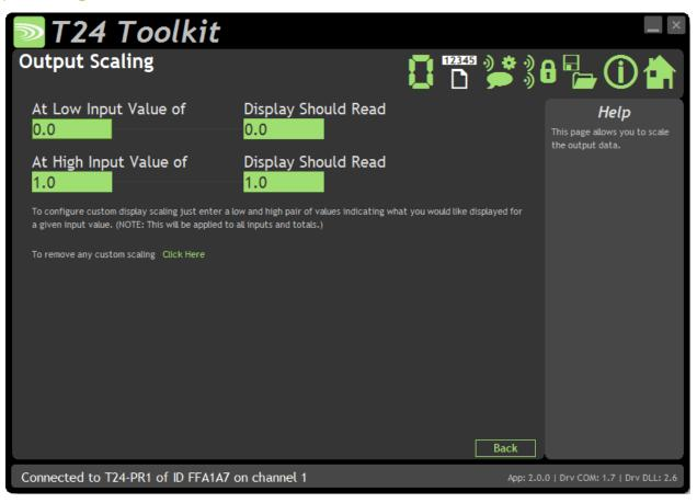
This page allows effective conversion between units. i.e. Although all modules supplying data are configured in kg you can get a printed output in lb.
