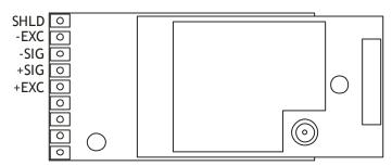
The resistance of the strain gauge can be between 85 and 5000 ohms. The T24-SA can support up to four 350 ohm strain gauges bridges attached in parallel (At the expense of reduced battery life).
