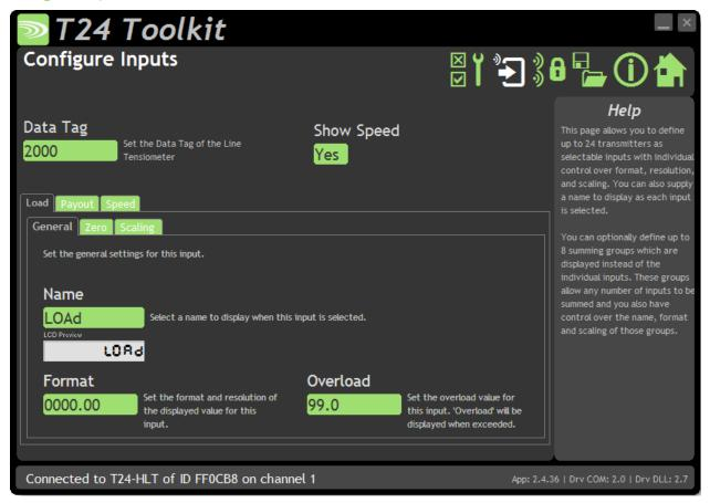
Here you can configure which transmitter is supplying data along with the configuration of the Load, Payout and Speed channels.
