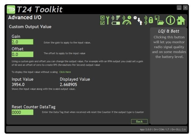
This module does not provide calibration, as such, because it is factory calibrated. However, on this page you can adjust the gain to provide different output types.
