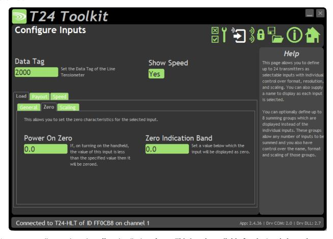
Here you can adjust settings that affect the display of zero. This is only available for the Load channel.
