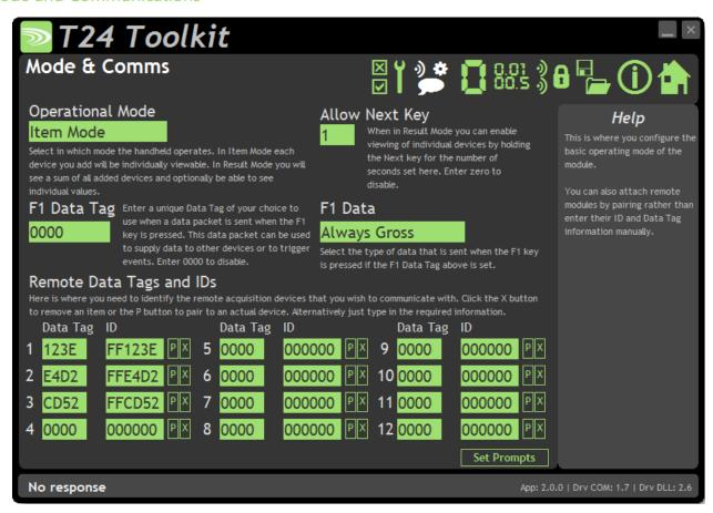
This page allows you to set the operational mode of the module and configure which external transmitter modules the handheld will connect to.
