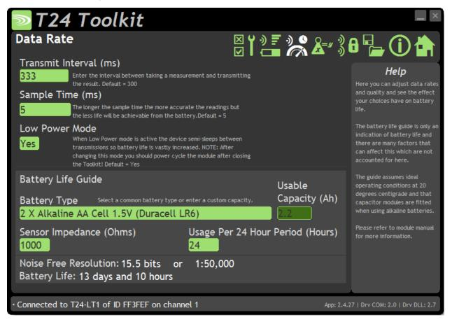
This page allows you to select the rate at which data is transmitted from the module and the quality. By selecting low power mode and entering some other information the toolkit will also give guides on achievable battery life. Note that the battery life calculator is assuming the best case scenario which is at 20 °C and that the battery has a suitable low internal resistance or that a suitable capacitor is fitted across the battery. See battery details in the Installation section.
