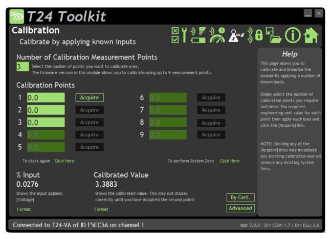
Here you can calibrate the transmitter module and set a system zero if required.
