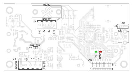
The interface can be selected from the DIP switches **SW1** as can baud rates for serial interfaces and the Address of the base station.
