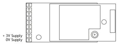
Connect to a 3 Volt power supply or batteries.
