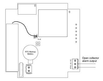
This is an open collector drive and can be used to operate alarms, klaxons etc.
