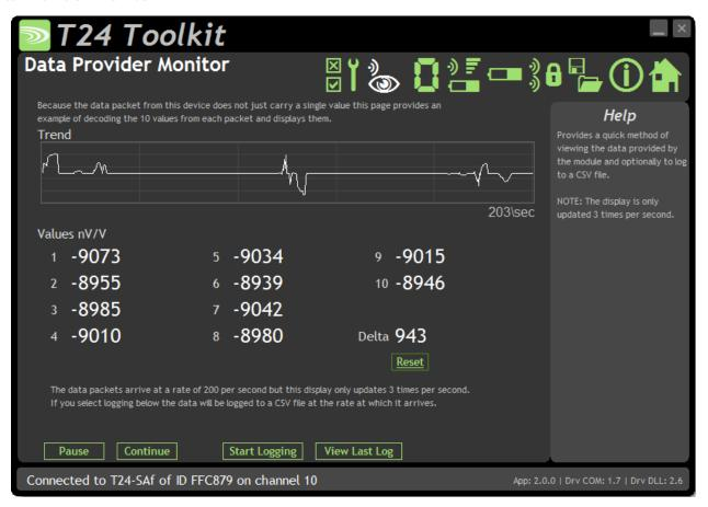
Because the standard data provider monitor does not decode correctly the multiple data packets from as T24-SAf this special page provides a trend chart and a view of all 10 readings contained in each packet. It also shows a delta value (Max – min) and allows you to log the data to a file.
