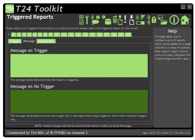
On the previous Trigger Tab you select whether the report is triggered transitionally or not. If triggered transitionally you can specify not only the message to send when the trigger test is true but also a message to send when the trigger test returns to false again.
