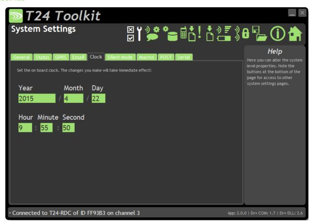
Here you can set the internal real time clock which is used to schedule the data collection and delivery.
