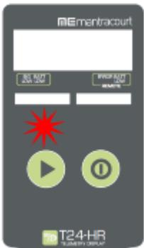
The handheld has the ability to configure a transmitter module to match the handheld's own radio channel and group key settings. Ensure that the transmitter module is unpowered for at least 10 seconds. Locate the upper left key by feeling for a slight bump on the label.
