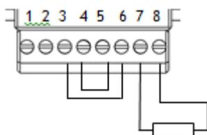
Strain Element in Tension
