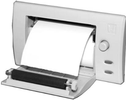
**4** Once the roll is fitted, close the door ensuring that the paper exits through the small gap at the top of the door and is not skewed.
