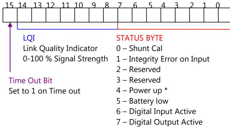
\* - This flag is set if the module has had power interrupted i.e. is running due to battery change
