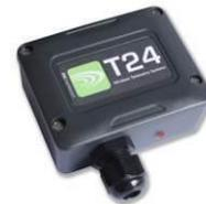
Resistance transmitter module mounted in medium weatherproof enclosure with battery holder for two AA batteries.
