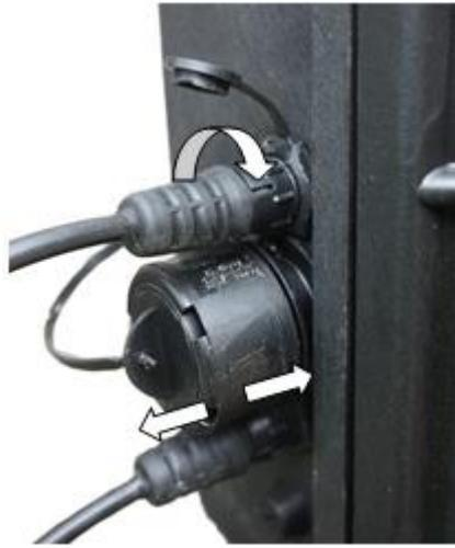
The PP1 110 Vac – 240 Vac input has a sealing cap for when it is not connected to the mains. The sealing cap is removed by pushing the outer sleeve towards the case and pulling the cap out.
