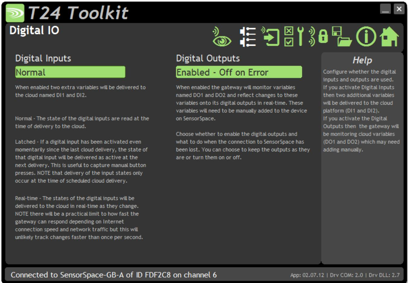
Here you can choose how to work with digital inputs and outputs..
