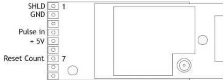
The 'Pulse in' input incorporates a pull-up resistor enabling a 'volt-free' contact to be used as the input source. This can take the form of a normally open or normally closed switch or relay contacts.
