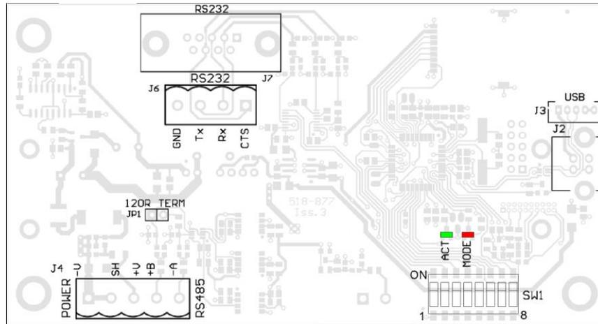
The interface can be selected from the DIP switches **SW1** as can baud rates for serial interfaces and the Address of the base station.
