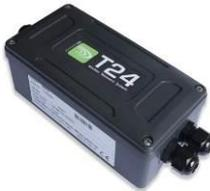
Voltage transmitter module mounted in large weatherproof enclosure with battery holder for two D cell alkaline batteries. Also has ability to be powered from external supply voltage.
