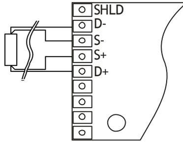
The four-wire resistance thermometer configuration increases the accuracy and reliability of the resistance being measured: the resistance error due to lead wire resistance is zero. In the diagram above a standard two-terminal RTD is used with another pair of wires to form an additional loop that cancels out the lead resistance. It provides full cancellation of spurious effects; cable resistance of up to 15 ohms can be handled.
