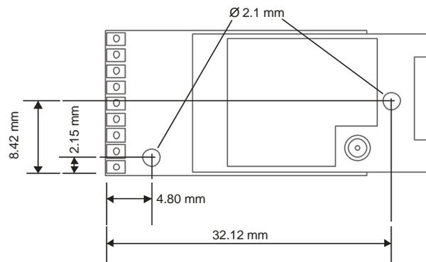
There are two holes available for mounting. The one nearest the connection pads can accept an M2 screw or American equivalent #0-80.
