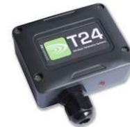
Voltage transmitter module mounted in medium weatherproof enclosure with battery holder for two AA batteries.
