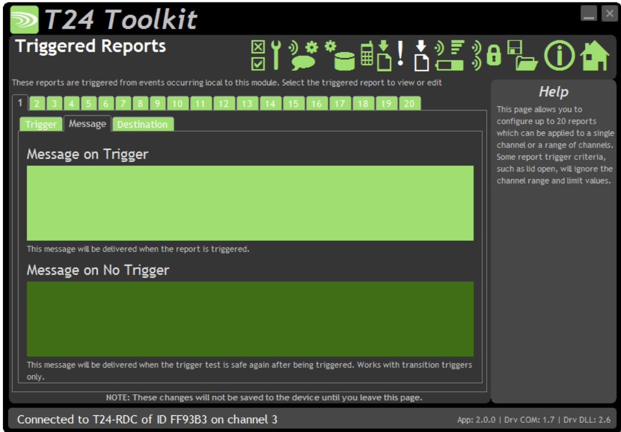
On the previous Trigger Tab you select whether the report is triggered transitionally or not. If triggered transitionally you can specify not only the message to send when the trigger test is true but also a message to send when the trigger test returns to false again. In the above example you can see that the No Trigger message is disabled because this is not a transitional triggered report.
