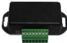
Pulse transmitter module mounted in small enclosure with screw terminals to connect external 3 V power supply.
