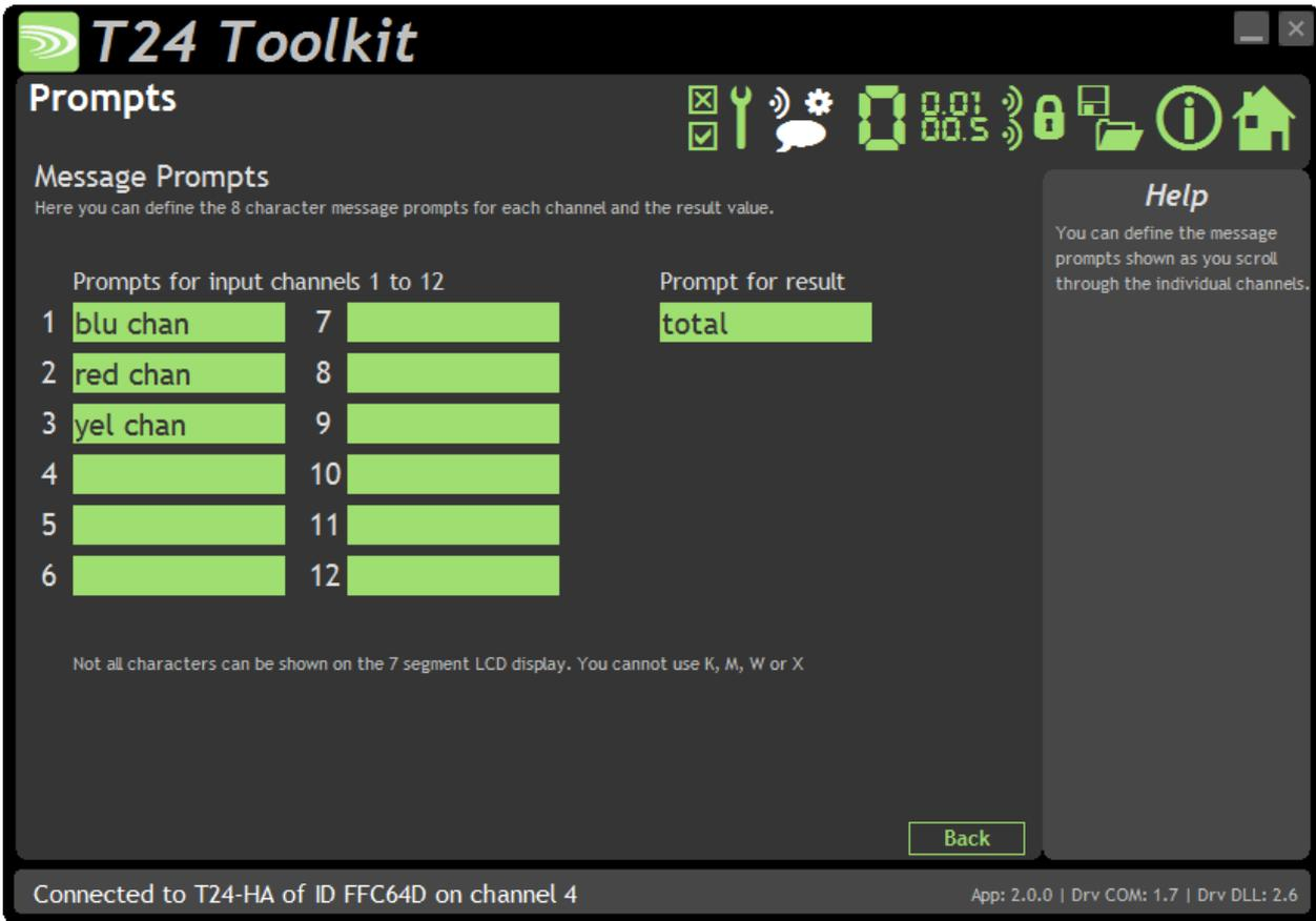
Here you can adjust the messages shown when switching between input channels in Item Mode..
