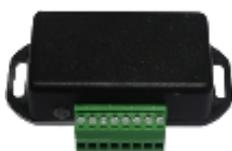
Current transmitter module mounted in small enclosure with screw terminals to connect external 3 V power supply.
