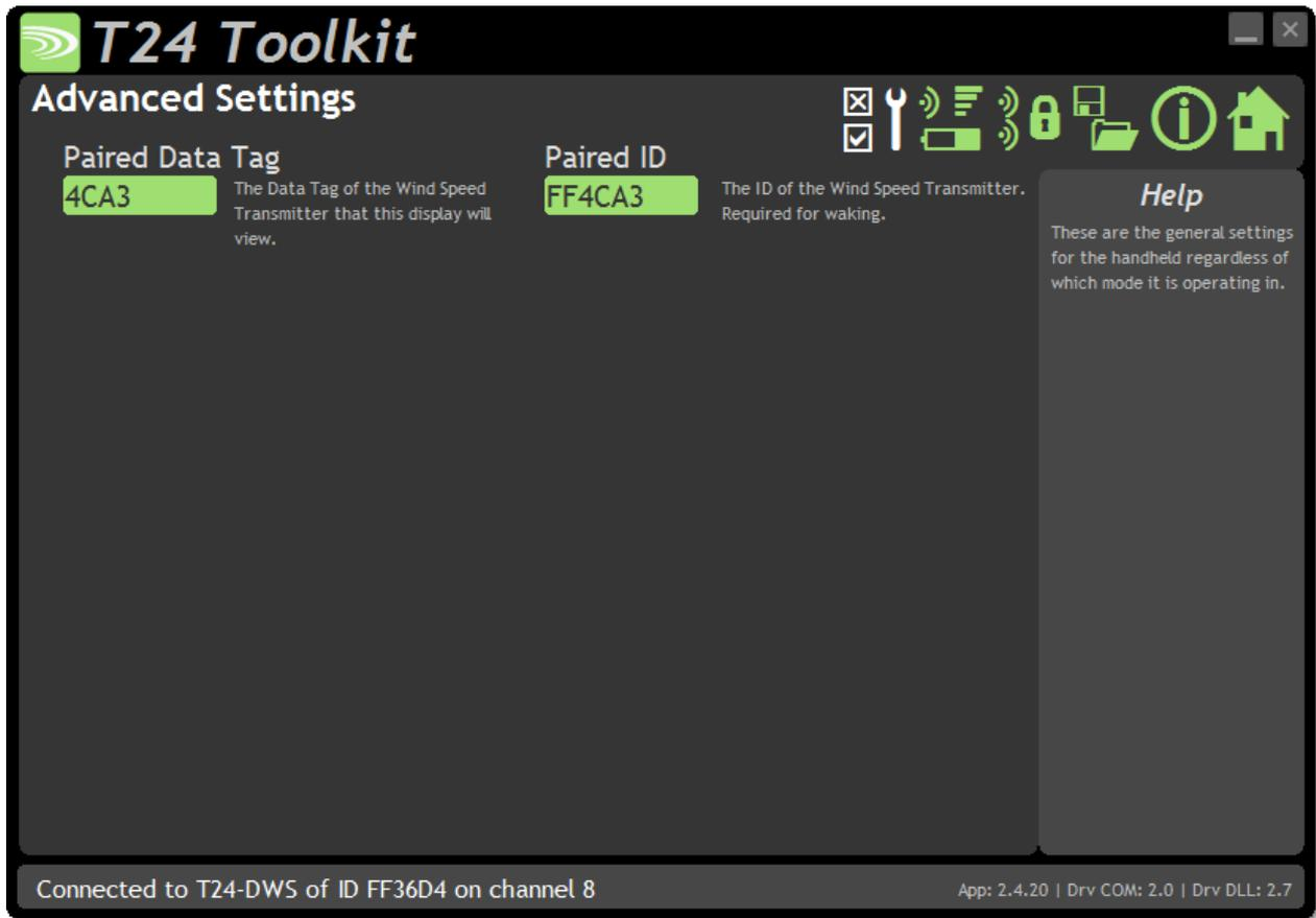
Here you can adjust the details of the transmitter to be connected with.
