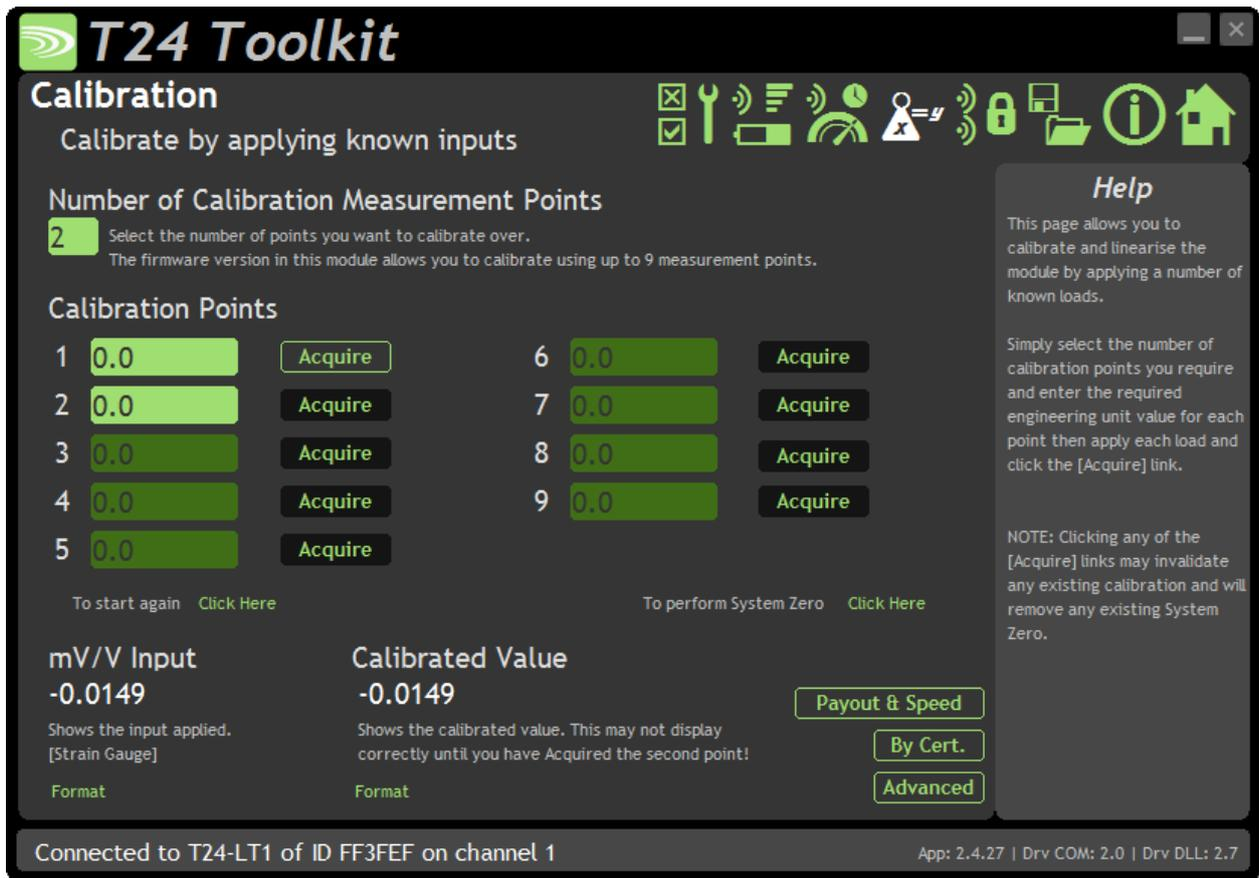
Here you can calibrate the transmitter module and set a system zero if required. This simple page allows semi-automated calibration where you can apply known inputs to calibrate. This calibration includes linearisation and is automatically applied. See later for **By Cert** and **Advanced** page where you can adjust individual gains and offsets.
