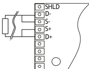
The simplest resistance thermometer configuration uses two wires. It is only used when high accuracy is not required, as the resistance of the connecting wires is added to that of the sensor, leading to errors of measurement. This configuration allows use of 100 meters of cable.
