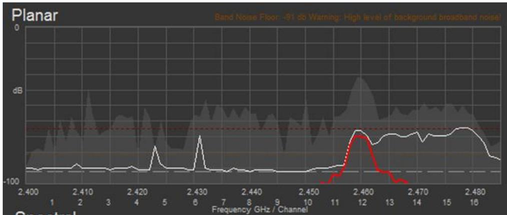
This shows how the display would look if the band noise floor slowly crept up. The red trace is only visible on channel 12 but other channels that were once OK (Having a very low minimum signal level) now have a viewable level of minimum signal noise. A double-click on the planar chart would reset the peak and minimum calculations so the minimum red trace would then follow the more recent higher noise floor.
