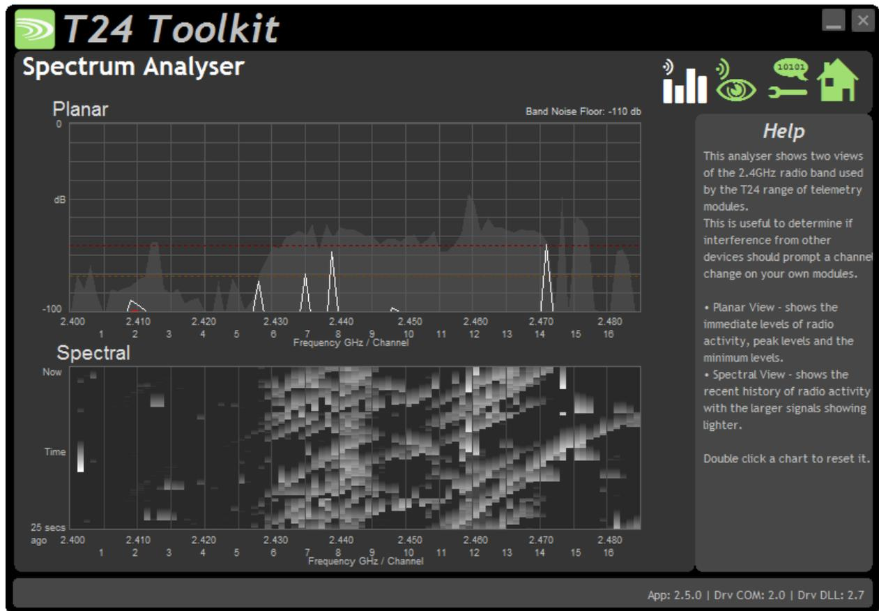
The spectrum analyser page is provided as a tool to use when conducting a site survey before installation, or to diagnose poor communications issues.
