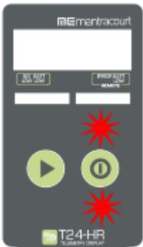
The handheld has the ability to perform a system zero on a remote transmitter module. This may be useful after installing new modules and enables system zero to be set without the need for a PC/laptop and T24 Toolkit.
