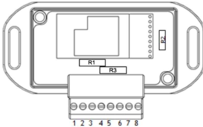
The T24-ACMm has the option for users to add up to three completion resistors, these can be used to enable the T24-ACMm to accept half and quarter bridge strain input when a strain transmitter module is fitted. The three completion resistors are located as shown below:
