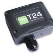
Pulse transmitter module mounted in medium weatherproof enclosure with battery holder for two AA batteries.
