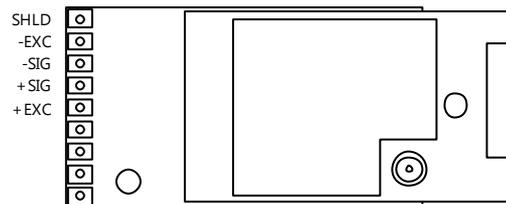
The resistance of the strain gauge can be between 85 and 5000 ohms. The T24-LT1 can support up to four 350 ohm strain gauges bridges attached in parallel (At the expense of reduced battery life).
