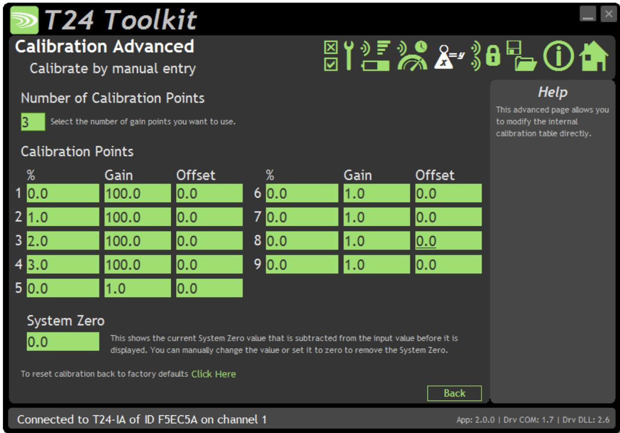
In some circumstances it may not be possible to apply inputs in which case the calibration can be entered manually.
