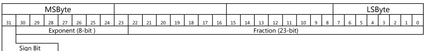
The byte containing the sign and exponent is sent first, with the LS byte of the mantissa being last. The value of the number is thus
