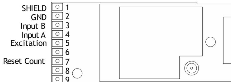
The 'Input A' input is used for Frequency, RPM, Interval, Counter, Digital State and Mark output types. This can take the form of a normally open or normally closed switch or relay contacts. The input resistor selection of pull up or pull down can be selected to suit the input.
