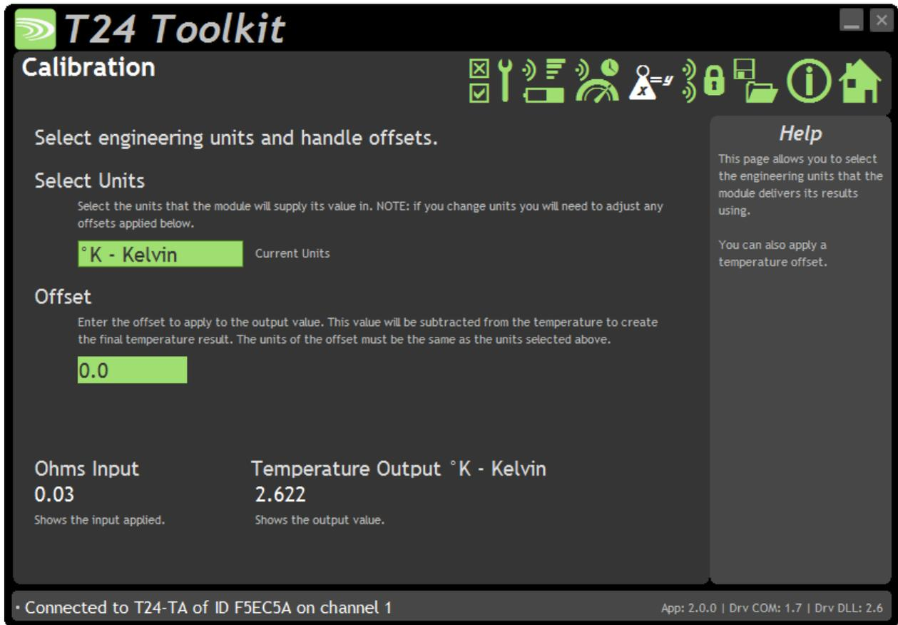
This module does not provide calibration, as such, because it is factory calibrated. However, on this page you can select the units and set an offset if required.
