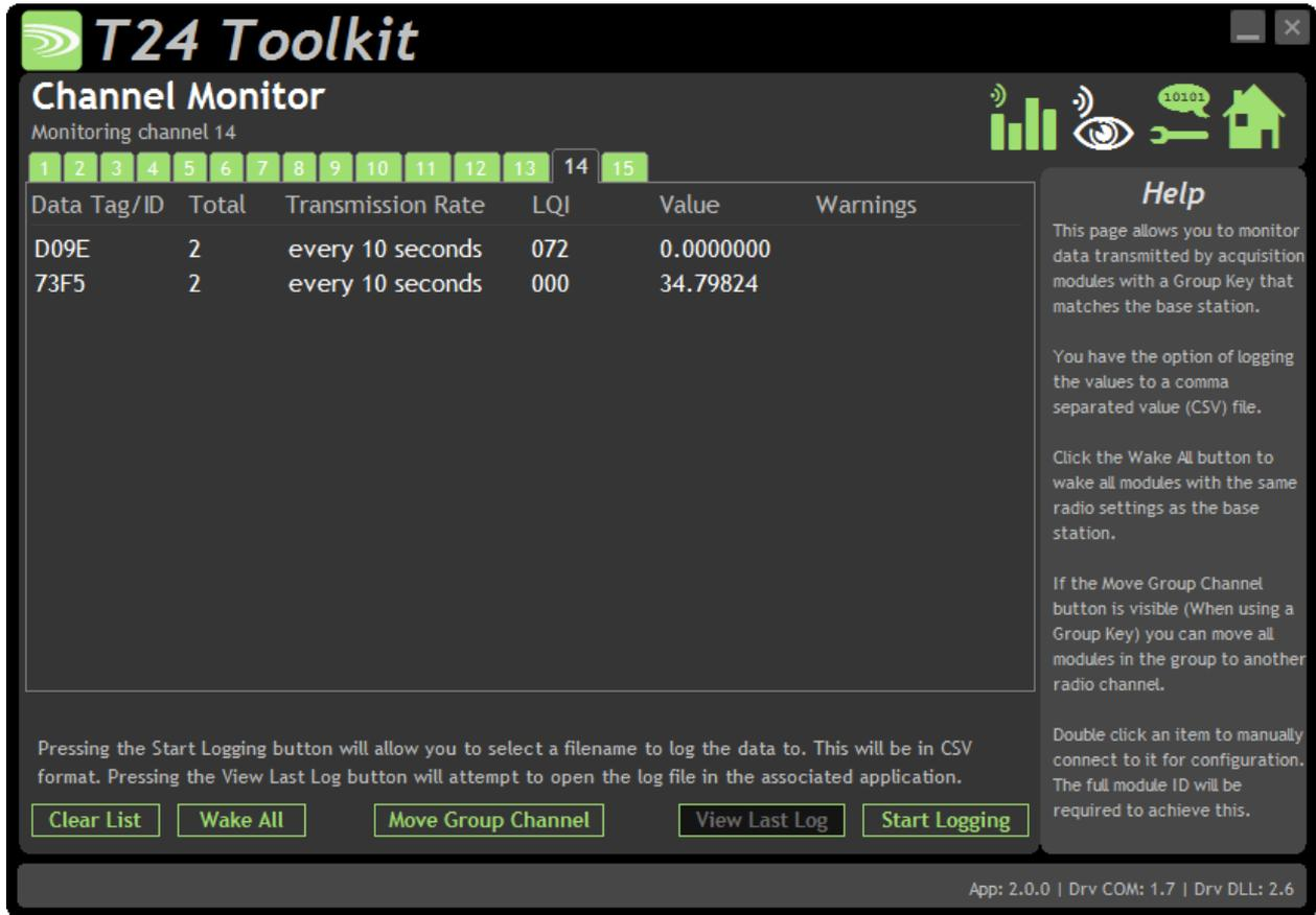
This page shows a summary of data sent by transmitter modules. You can see the Data Tag of transmitted messages along with the total number of messages received, the transmission rate, link quality, data value and any error messages. Some base stations can also list modules that are sleeping. These will show an ID instead of a Data Tag.
