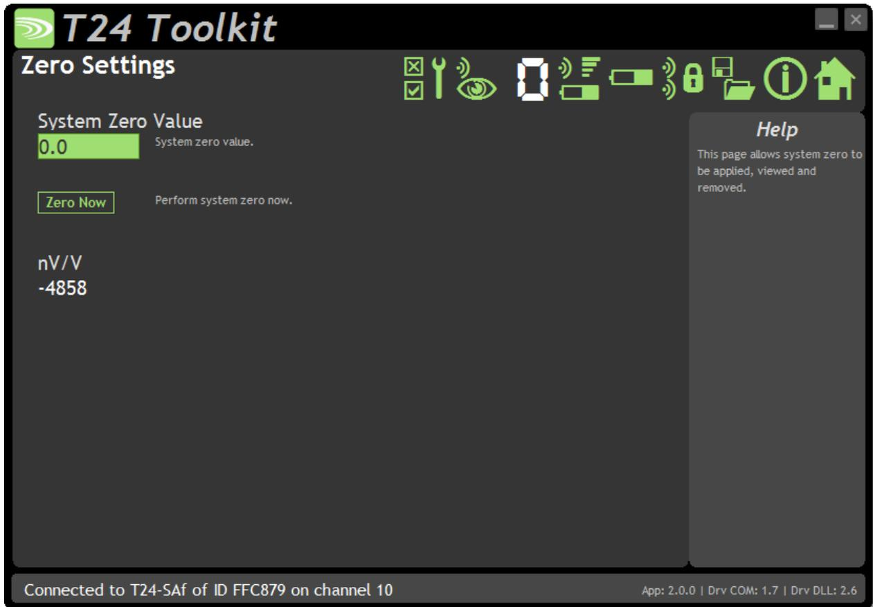
Although there is no calibration functionality in the T24-SAf there is the ability to zero the output value.
