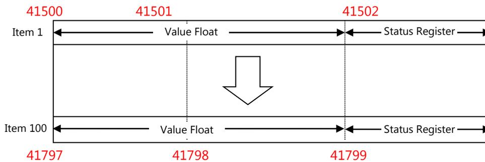
When reading registers containing the floating point data the register pairs must be read at the same time otherwise incorrect values could result because of partial updates during reading.
