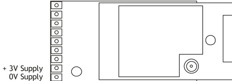
Connect to a 3 Volt power supply or batteries.
