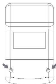
Once the battery compartment has been removed this gives access to two further screws which can be removed (along with the two at the top end) to allow the entire case to come apart. This gives access to the legend channels where cardboard legends can be slipped in behind the transparent label windows where supported. Note that the top two screws will have rubber 'O' rings on them. These rings are an integral part of the sealing mechanism.
