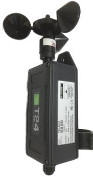
Wind speed transmitter module mounted in large weatherproof enclosure with battery holder for two D cell alkaline batteries. Also has ability to be powered from external supply voltage.
