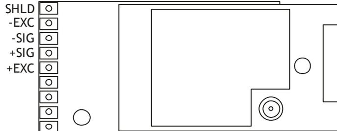
The resistance of the strain gauge can be between 85 and 5000 ohms. The T24-SA can support up to four 350 ohm strain gauges bridges attached in parallel (At the expense of reduced battery life).
