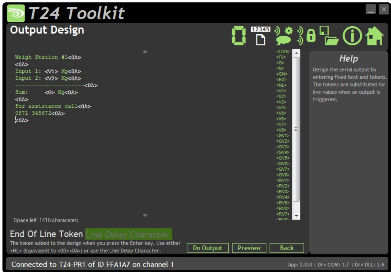
This is where you define the actual printed output based on free text and tokens. Tokens are special codes contained within angled brackets <token> which have special meanings and are converted to actual values once an output is triggered. See list of tokens at the bottom of this section.
