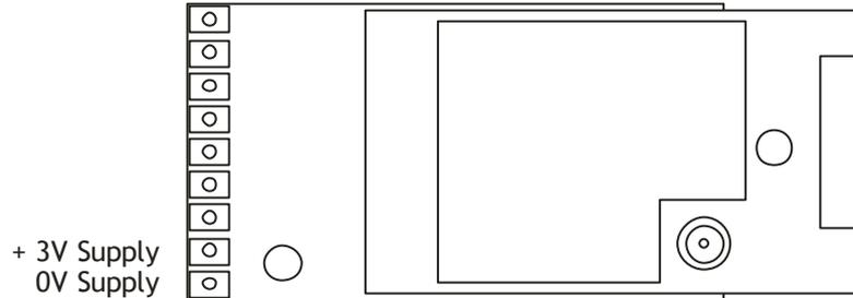
Connect to a 3 V power supply or batteries.
