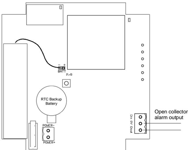
This is an open collector drive and can be used to operate alarms, klaxons etc.
