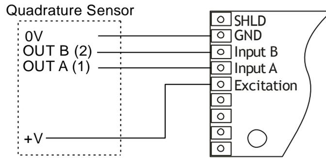
Onboard resistor configured to suit sensor and suitable excitation voltage selected
