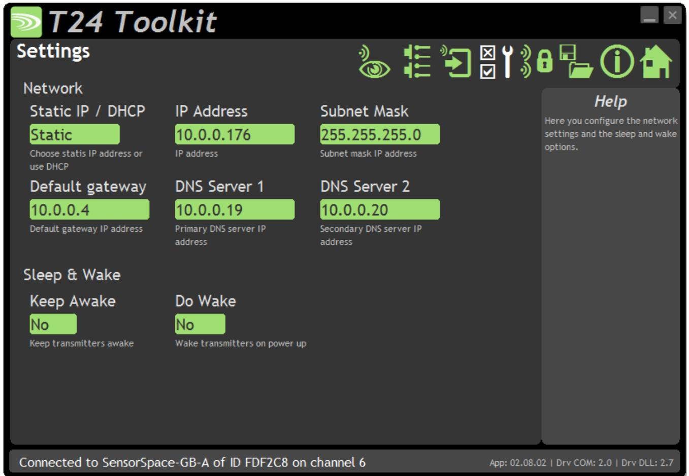
This page allows you to configure the Ethernet network settings and the wake functions.
