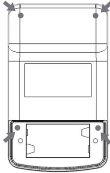
When the case comes apart be careful of any wires running between the two case halves.
