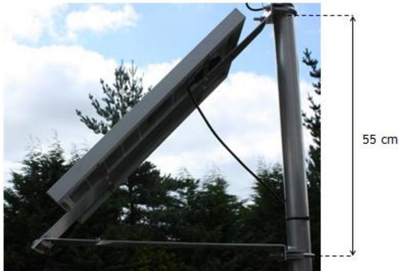
When positioning the solar panel it should always face true south if you are in the northern hemisphere, or true north if you are in the southern hemisphere. True north is not the same as magnetic north. If you are using a compass to orient your panels, you need to correct for the difference, which varies with location. Search the web for "magnetic declination" to find the correction for your location.
