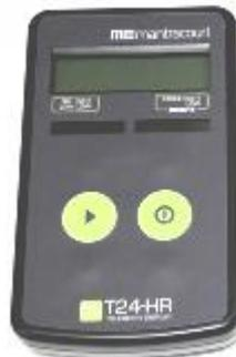
Handheld display for unlimited number of transmitter modules in a robust weatherproof enclosure.
