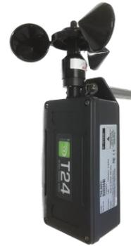
Wind speed transmitter module mounted in large weatherproof enclosure with battery holder for two D cell alkaline batteries. Designed for pivot mounting to moving booms.
