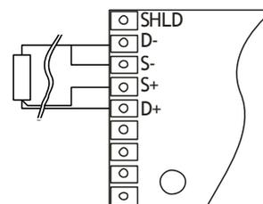
In order to minimize the effects of the lead resistances, a three-wire configuration can be used. Using this method the two leads to the sensor are on adjoining arms. There is a lead resistance in each arm of the bridge so that the resistance is cancelled out, so long as the two lead resistances are accurately the same. This configuration allows up to 600 metres of cable.
