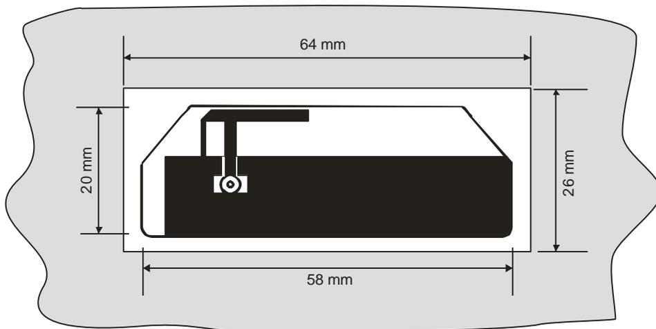
The antenna feeder cable, or any other cables or wires, must not be routed over or near the cross hatched area shown below as this will affect range.
