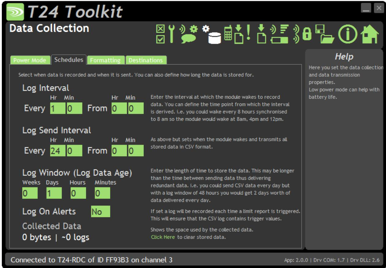
This tab sets the intervals at which data is collected and at which the CSV data is transmitted. This has an effect on battery life as in Low and Ultra Low Power modes the Log Interval determines how often the module wakes from a very low power sleep mode. See Battery Life section
