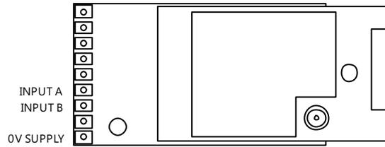
The quadrature input sensors A and B should be mounted so that the activation zones (Whether optical or magnetic etc) cover both A and B inputs simultaneously as rotation occurs.
