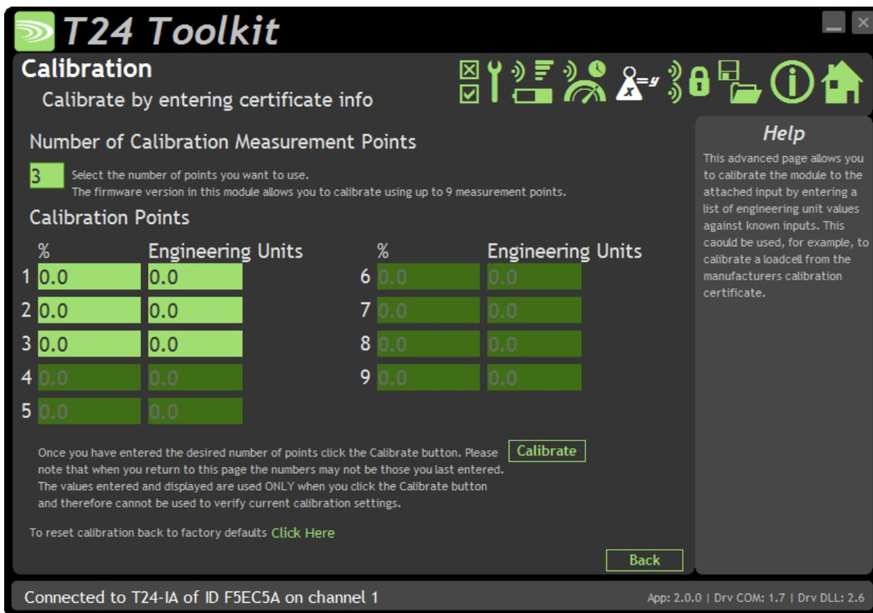
In some circumstances it may not be possible to apply inputs in which case the calibration can be entered manually from a calibration table.
