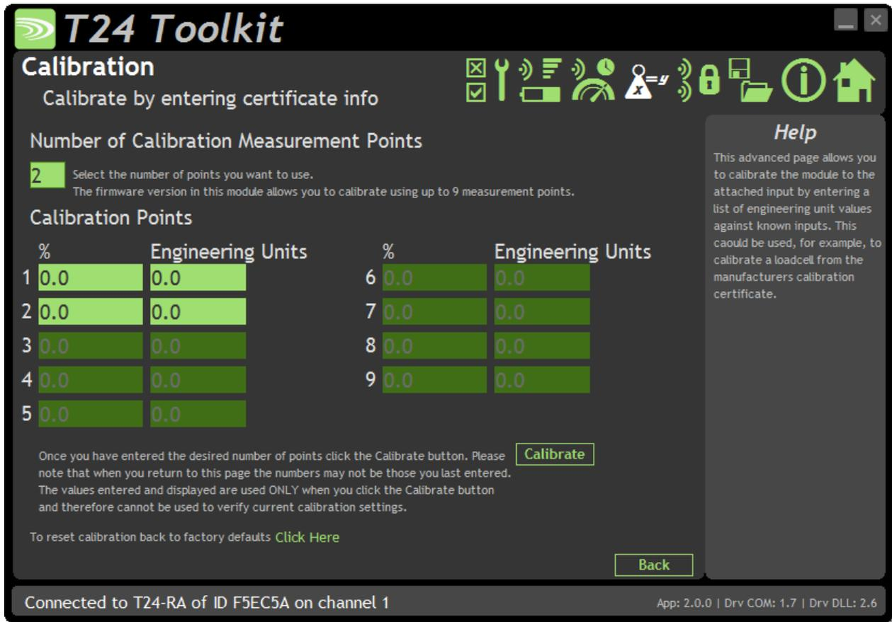
In some circumstances it may not be possible to apply inputs in which case the calibration can be entered manually from the calibration table or certificate without ever having to connect the input.
