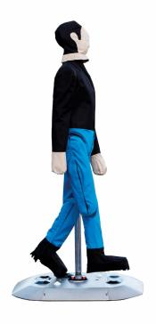
The Soft Pedestrian 360 from DRI is the next generation of articulated surrogate pedestrian target, bringing a whole new level of realism and vehicle protection to VRU testing.
