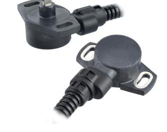
The SRH301 and SRH302 range of shaft-operated Rotary Position Sensors offers the optimal combination of performance, safety and cost. The sensor utilises proven Hall-effect, sensing technology in a low-profile (17.3mm) housing with integral magnet.
