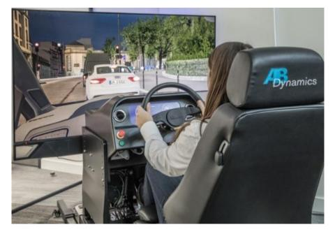
The static simulator from AB Dynamics is a class-leading solution that takes components from AB Dynamics' proven third-generation simulator to provide a cost-efficient way to reduce the cost and time of automotive system development through DiL simulation.
