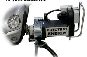
"A unique, all-purpose chassis dynamometer for special and general powertrain testing"
