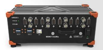
DEWESoft® introduces the MINITAURs, fully packed with the latest technology. Based on the SIRIUS® DUALCOREADC® technology with amazing dynamic, it offers eight universal analogue input channels and at the same time eight Supercounters® plus 1 CAN port for automotive applications.
