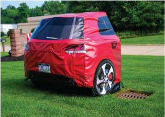
The Moshon Data Vehicle Target Foam is fully compatible with the Flex-Moshon towing system.
