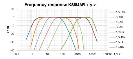
The HP filter of **velocity** sensor types has a stopband attenuation of -50 dB/decade, the LP filter has a stopband attenuation of - 40 dB/decade.
