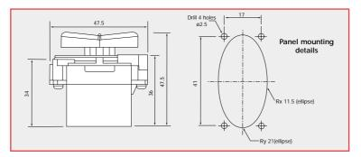
The recommended panel thickness is 3mm. The O ring supplied must be used to seal the JC030 rocker assembly to the mounting panel to enable IP60 protection. Supplied with 4 x panhead Pozidrive self tapping screws for mounting to panel.
