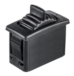
The JC050 is a roller for use in joystick grips and other in-cab human-machine interfaces. A robust, return-to-center mechanism provides movement over a range of ±37°, with the thumbwheel having an option of a lever profile to ease operation. A compact mechanical design means the required under-panel space is just 23mm.
