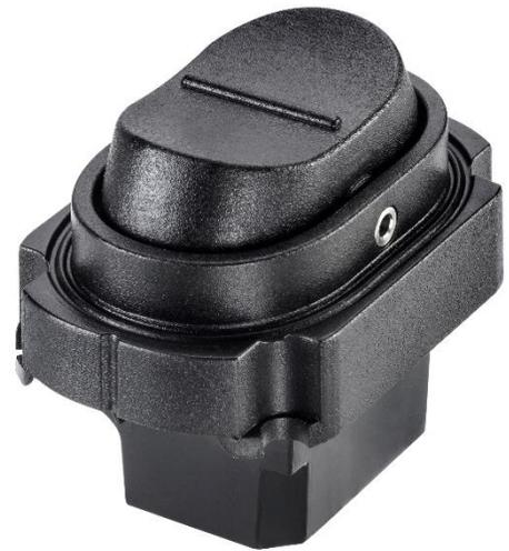
The JC040 is a proportional rocker for use in joystick grips and other in-cab human-machine interfaces. Two robust, return-to-center operating options are available: a  $\pm 25^\circ$  movement from center; or a  $\pm 20^\circ$  movement with an over-press feature, which can be included in both directions of movement or just one, used to indicate a different mode of machine operation. In all versions, a compact mechanical design means the required under-panel space is just 21mm.
