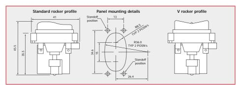
The recommended panel thickness is 3mm. The O ring supplied must be used to seal the JC025 rocker assembly to the mounting panel to enable IP65 protection.
