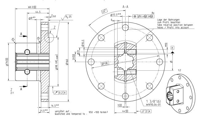
Profile sleeve 6 teeth (1 3/8''),  $\leq 5000$  Nm continuous dynamic load
