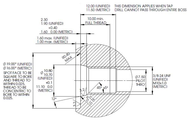
\* IF FACE OF PORT IS MACHINED DIMENSIONS Ø19.00 x 1.6 max (UNIFIED) /Ø16.00 x 1.00 max (METRIC) NEED NOT APPLY AS LONG AS R0.2/0.1 IS MAINTAINED TO AVOID DAMAGE TO O-RING DURING INSTALATION.
