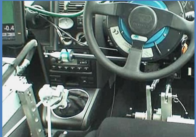
Prototype GR in operation with Driverless Test System
