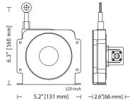
A perfect solution for both OEM and single-piece user, this string pot provides an economically priced CANopen sensor for 80-inch and 120-inch stroke range applications. This sensor is constructed with a rugged polycarbonate enclosure, a stainless steel mounting bracket and universally accepted M12 connector for operation in both outdoor or factory dry environments. For the OEM, customized options are available.
