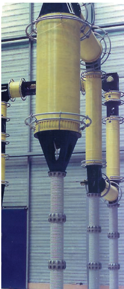
Fig. 23 Reactor bank for the voltage circuit for synthetic testing of circuit breakers; 32 kA peak to peak, 0,318 mH to 353,6 mH, up to 1600 kV BIL
