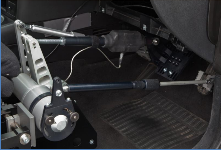
Under-seat pedal actuators (throttle, brake and clutch)
