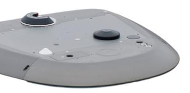
The LaunchPad Spin is the ADAS target platform that brings new levels of manoeuvrability to VRU testing. Its turn-on-the-spot, single wheel steering gives it the ability to rotate 360 degrees in an instant, so your testing can closely replicate the rapid changes in direction that are common to real-world pedestrian behaviour. Plus, its top speed of 30km/h also makes it capable of testing scenarios involving cyclists and e-scooters.
