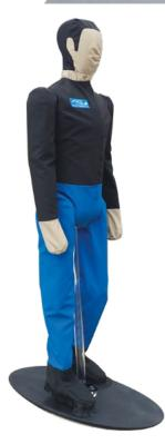
The Soft Pedestrian 360<sup>™</sup> from DRI is the next generation of articulated surrogate pedestrian target, bringing a whole new level of realism to VRU testing.
