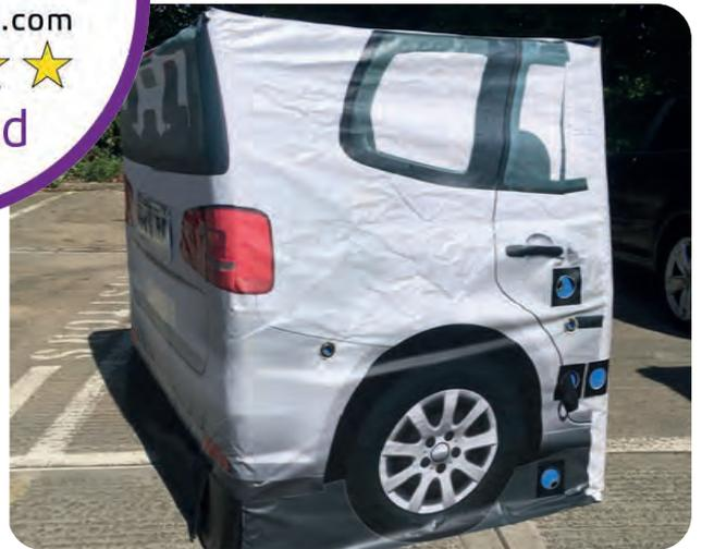
The Moshon Data EuroNCAP Vehicle Target (EVT) was developed to simulate the rear end of a standard production car and is suitable for RADAR, LiDAR and camera based systems.
