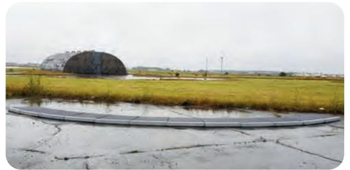
Moshon Data has designed and developed foam pavements / sidewalks in straight and curved sections to create configurable junction scenarios including Euro NCAP Car to Pedestrian Turning Adult.
