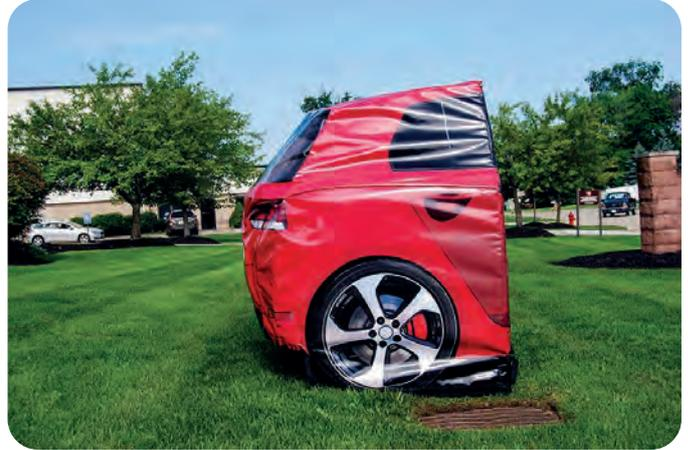
The MD-VT F is a lower cost, foam version of the official Euro NCAP Vehicle Target (EVT). It is designed to the same specifications as the Euro NCAP target and intended for development work. Being a cheaper substitute for the EVT means vehicle manufacturers and test facilities can purchase multiple vehicle targets and increase the number of tests.
