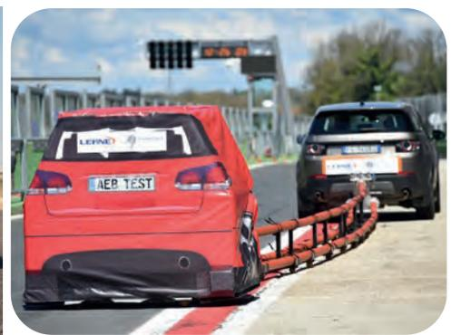
The Flex-Moshon towing system is designed to tow a balloon car during Autonomous Emergency Brake (AEB), Forward collision warning (FCW) and other ADAS tests.
