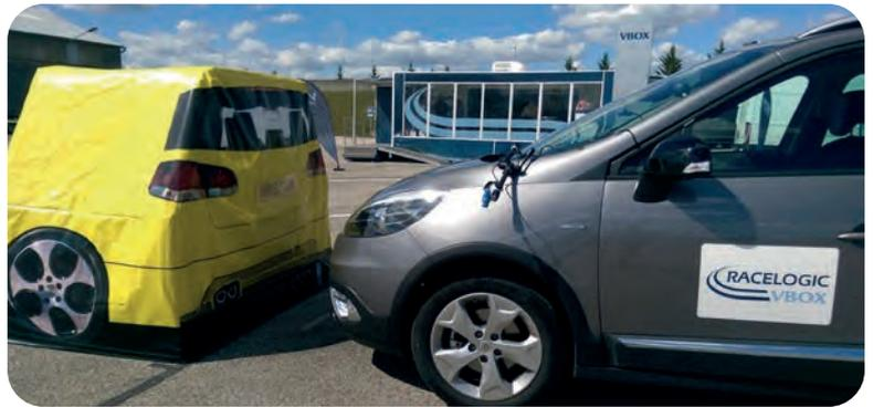
The MD-VT and MD-VT L (Large) is an inflatable, lower cost version of the official Euro NCAP Vehicle Target (EVT). It is designed to the same specifications as the Euro NCAP target and intended for development work. Being a cheaper substitute for the EVT means vehicle manufacturers and test facilities can purchase multiple vehicle targets and increase the number of tests.
