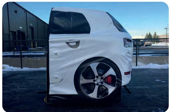
Ideal for end of line production use - does not require regular maintenance to keep inflated, conforms to ISO standard! Sensor specific recognition properties as shown in document ISO 19206-1:2018(E) Annex B (Page 10)
