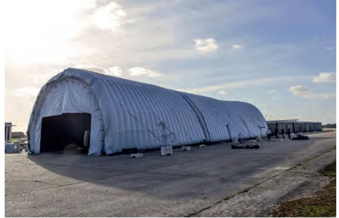
This is a unique solution for testing ADAS sensors in the dark. Exclusively available from Moshon Data, the sectional Inflatable Tunnel can be configured in various options.
