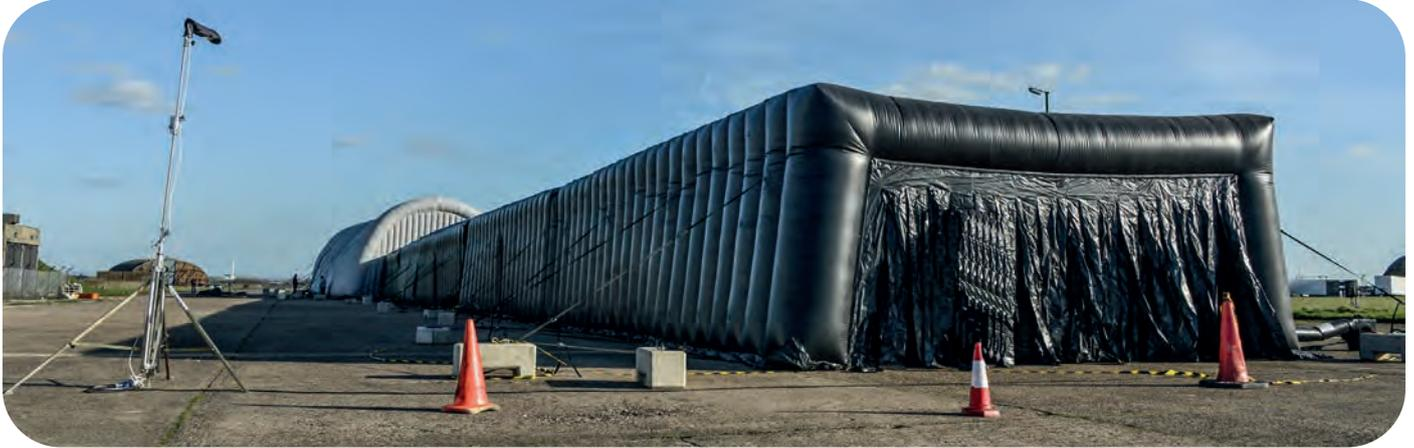
This is a unique 300ft (91m) long tunnel for testing ADAS sensors in the dark. Exclusively available from Moshon Data, the night vision tunnel provides interior light blocking to assist with the development of night vision assist technology. The tunnel consists of six 50' long connecting sections, five emergency exits/exit lights every 50' and three 5000 CFM exhaust fans to clear the air after every run through. The tunnel is suitable for AEB and VRU tests.
