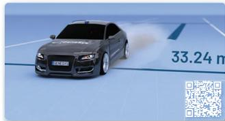
The ADMA-Speed enables unmatched accurate and simple leading measuring solution to perform brake tests and tire inspections. ADMA-Speed is a tried and tested variant of our Automotive Dynamic Motion Analyzer (ADMA), which provides reliable, accurate (up to 0,05 m RMS) and easy usable measurement data, compensation of the vehicle pitch during braking process, easy and quick installation & drift compensation at standstill.
