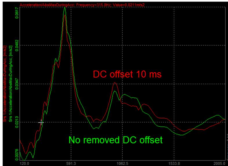
**Noise floor** (in milliseconds) will calculate the noise floor of the input time signal. The noise floor will be calculated the defined time interval behind the position of the first cursor.
