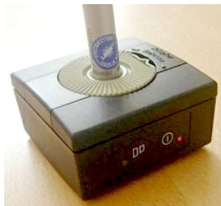
Illustration 7: Calibration with Sound Calibrator (1 Pa = 94 dB at 1 kHz)
