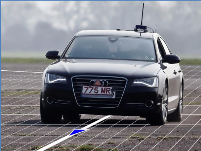
Driverless testing using path-following software
