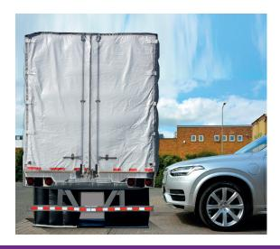
A combination of inflatable and foam components with high-tech fabrics and complex construction aimed at replicating the shape of a real semi-truck trailer whilst maintaining the correct radar signatures required for high-fidelity simulation.
