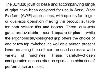
Non-contacting, Hall-effect sensing technology ensures smooth operation and a long life – in excess of 6 million operating cycles – while dual electrical outputs on each axis, plus a center-reference signal, enhance overall system safety. The range of the
