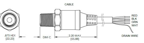
Digital Output Connection (Cable Type)
