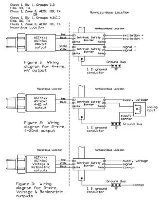
Models AST4400, AST44LP, AST4500, AST4510, AST4520, AST4530 Class I, Div. I, Groups C,D; EXIa IIB, T4; Class I, Zone 0, AEXIa IIB, T4 Vnax = 28Vdc
